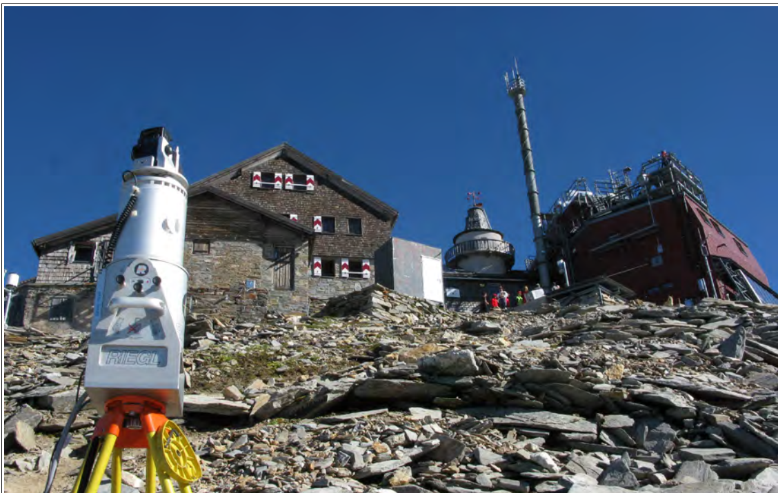
Fig. 2: The Riegl 3D-LaserScanner in operation at the ZAMG Sonnblick observatory, Austria 2010
