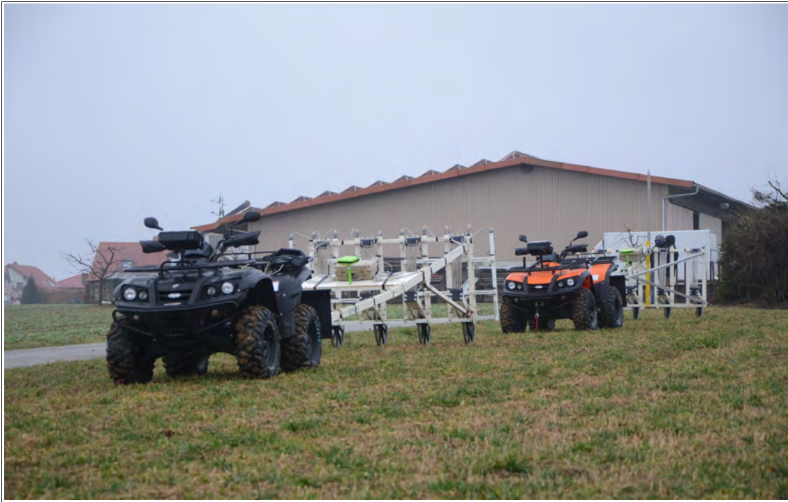
Fig. 4: The two Foerster Fluxgate magnetometer systems in Schalkstetten, Germany 2011.
