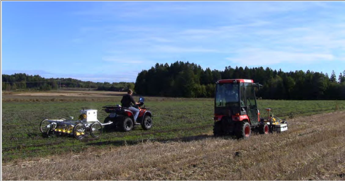
Fig. 3: MIRA and SPIDAR GPR systems in operation in Vestfold county, Norway 2010
