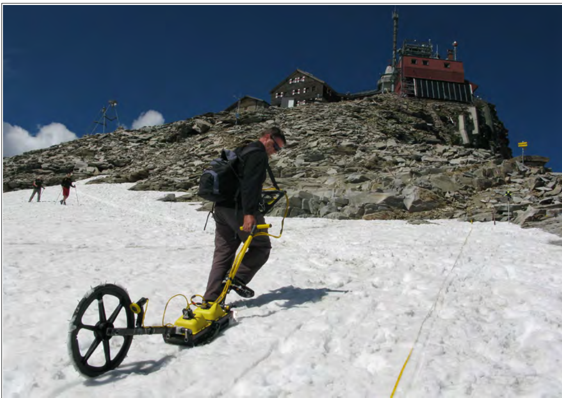
Fig. 13: GPR prospection in 3050 m above sea level at the Sonnblick, Austria 2010
