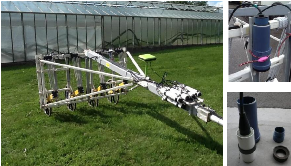
Motorized 6-channel Caesium magnetometer system
