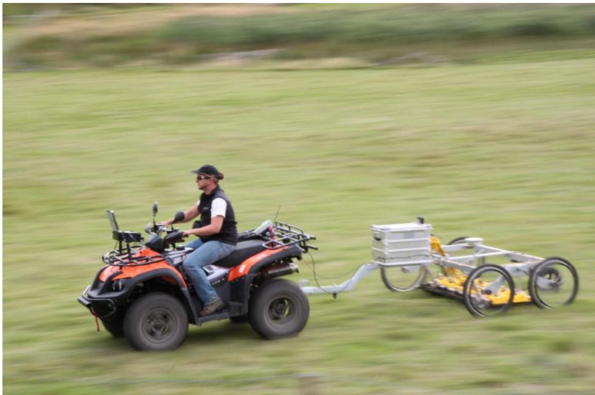
Motorized SPIDAR GPR in operation
