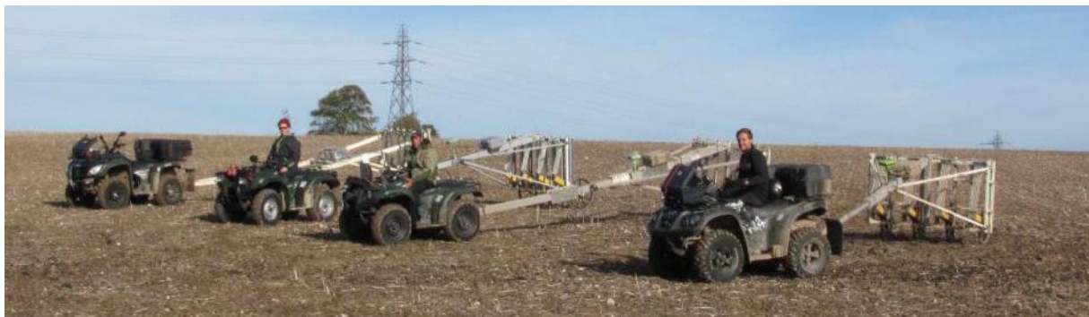
Motorised LBI ArchPro fluxgate magnetometer systems in operation at Stonhenge
