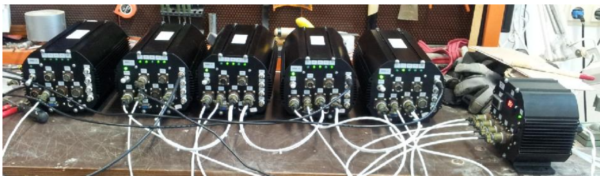
Array of five A/D converters for a 20 channel Caesium magnetometer system
