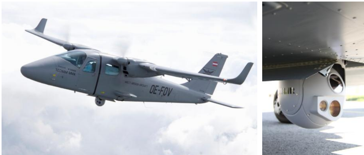
The versatile main airborne platform of LBI ArchPro partner ABT with integrated airborne laser-, hyper-spectral- and thermal-scanners.
