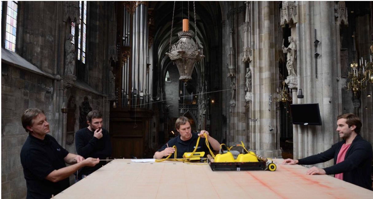
Fig 19: GPR survey in St. Stephen's Cathedral, Vienna
