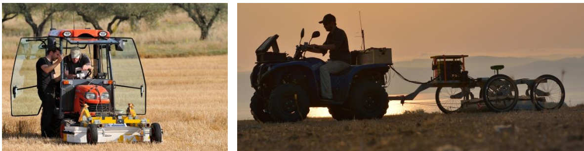
Fig. 24: GPR survey at Bisenzio with the 16-channel MIRA system (left) and the 6-channel SPIDAR system (right).
