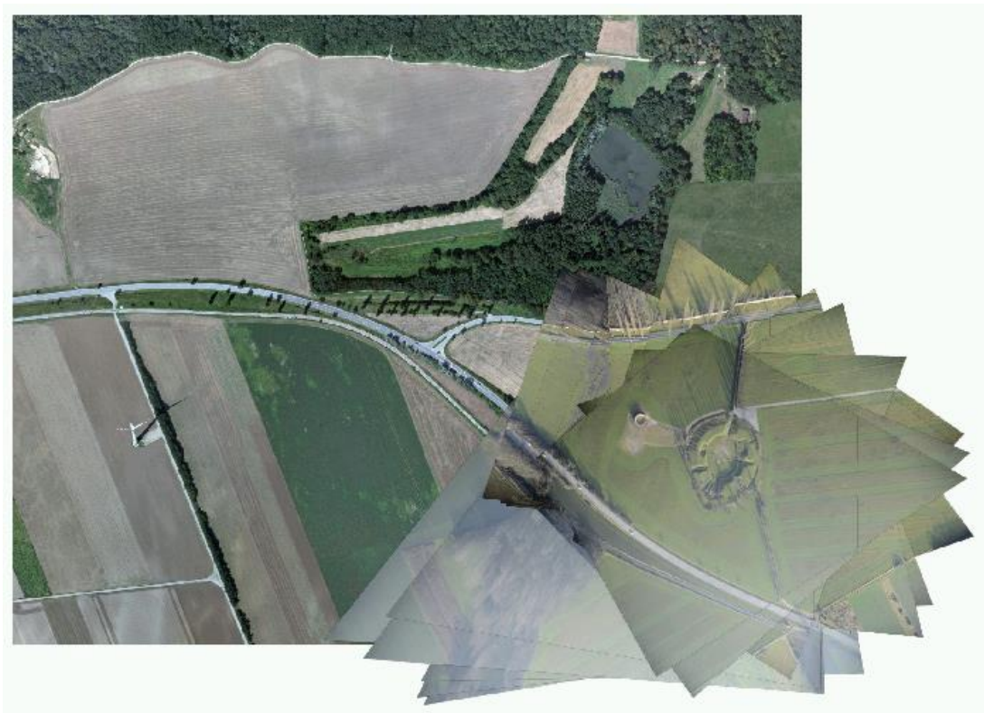
Fig. 11: Result of automated transformation images on a plane surface using the GPS and IMU data.
