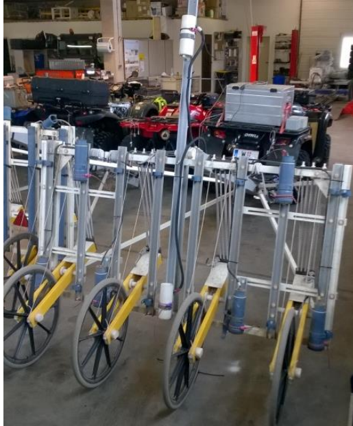
Fig. 2: Caesium magnetometer cart with sensors placed at three different heights above ground.
