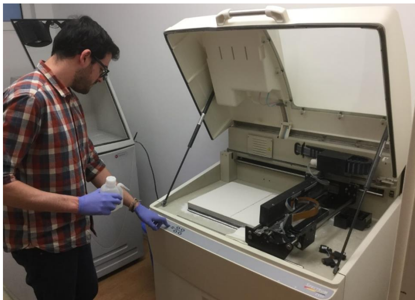
Fig. 3: Juan Torrejón Valdelomar operating the Z Cooperation SPECTRUM Z TM 510 3D gypsum powder printer. The model cleaning unit can be seen in the background.
