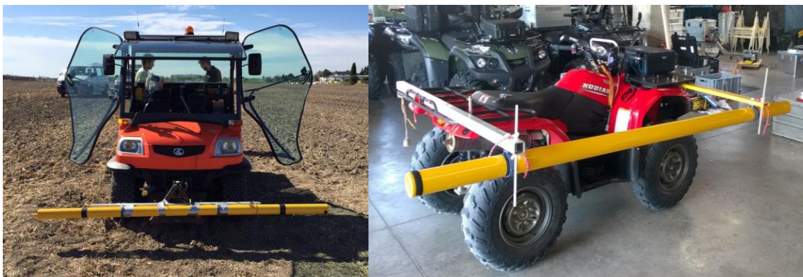
Fig. 12: The DualEM 21HS mounted in front of the Kubota tractor and alongside a Quad bike for the survey in Bisenzio.
