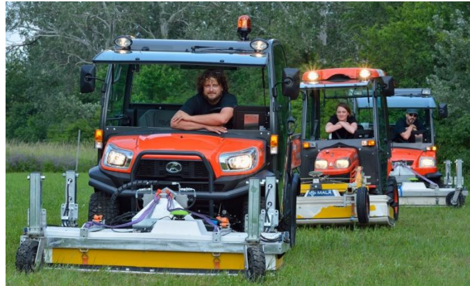
Fig. 1: The three 16-channel MIRA systems now in use within the LBI ArchPro family.
