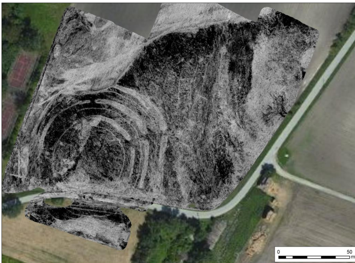
Figure 14: Depth slice 40-100cm measured with the MIRA 2 ground penetrating radar array at the Middle Neolithic site Velm, NÖ.
