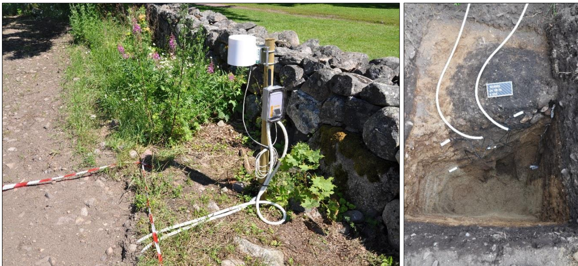
Figure 20: Monitoring station at the archaeological park Borre and the positioning of sensors in one of the re-excavated large postholes of one of the Viking Age hall buildings.
