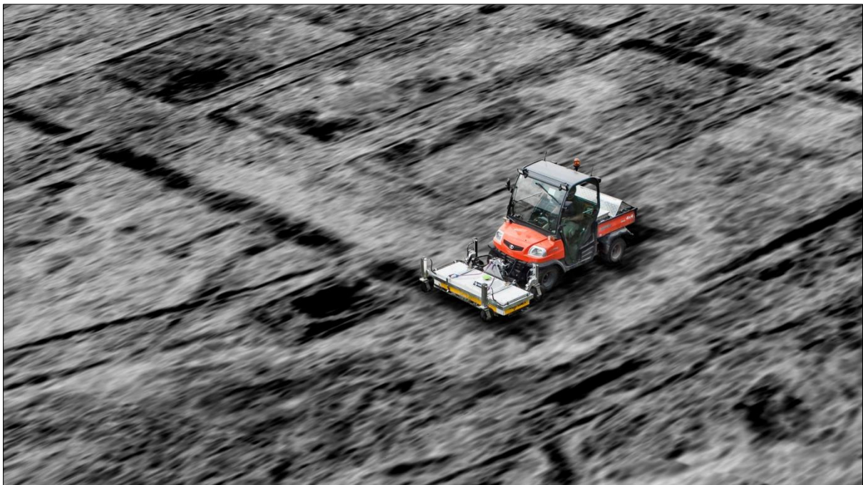
Figure 7: MIRA ground penetrating radar array placed on top of a data visualisation.
