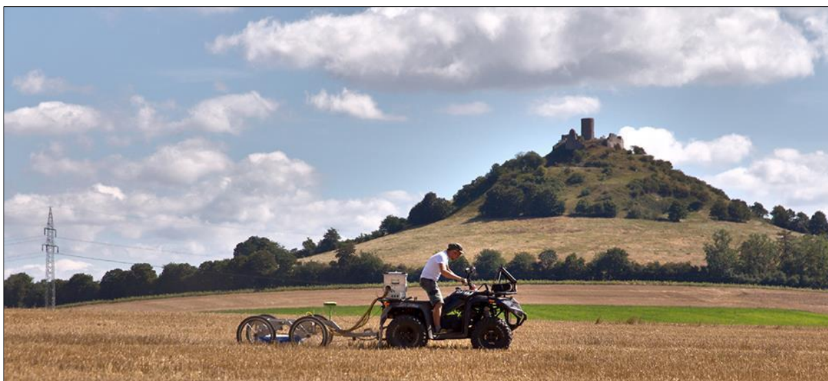
Figure 21: Ground penetrating radar survey using a SPIDAR 500 MHz system at Desenberg, Westfalia.
