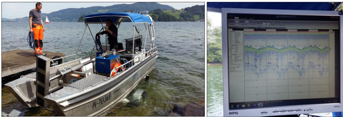
Figure 12: Test survey with the Innomar SES-2000quattro 4-channel sediment sonar in very shallow water at Lake Mondsee in May 2016.
