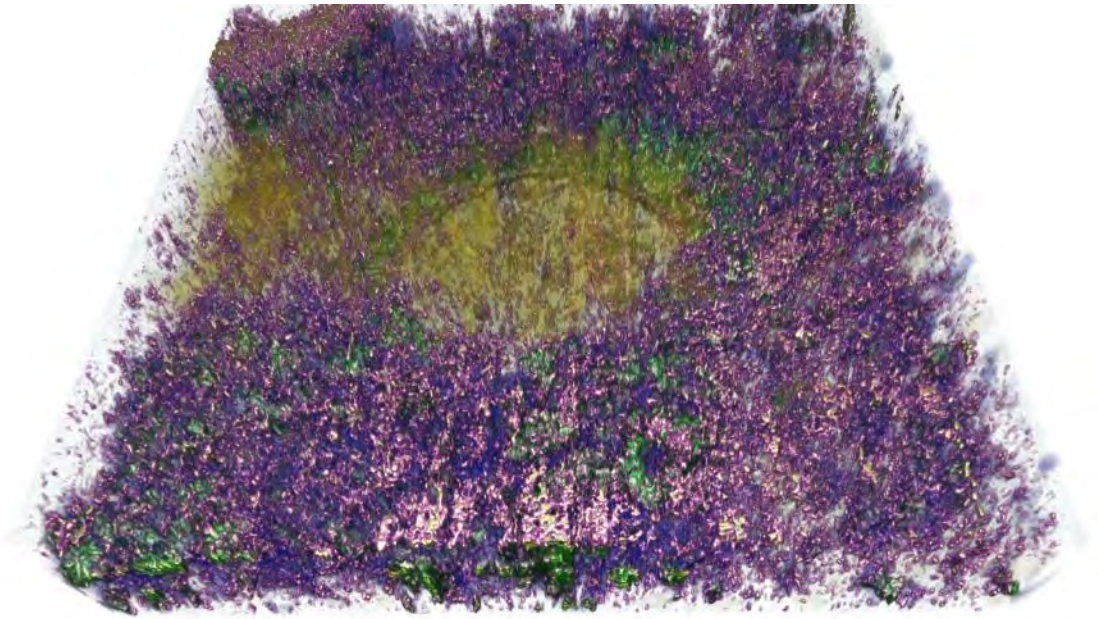
Fig. 29. GPR visualisation from the Stonehenge dataset. The new scaling feature for the GPR visualisation – in this example the depth is scaled by a factor of 2.5 - better depicts the circular ring-shaped geological structures.
