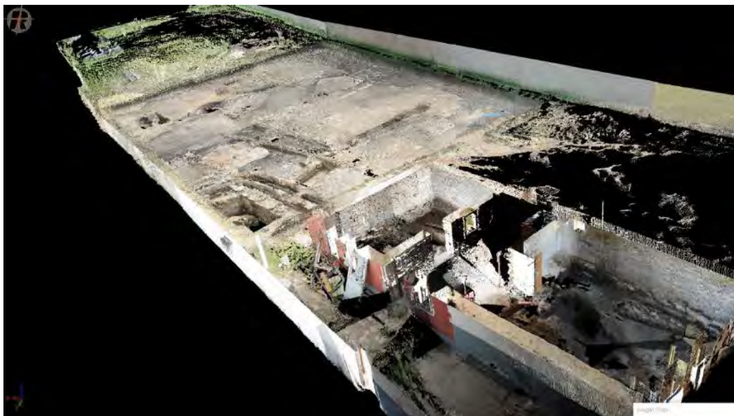
Fig. 19: Perspective view of the texturized point cloud, Müllendorf.
