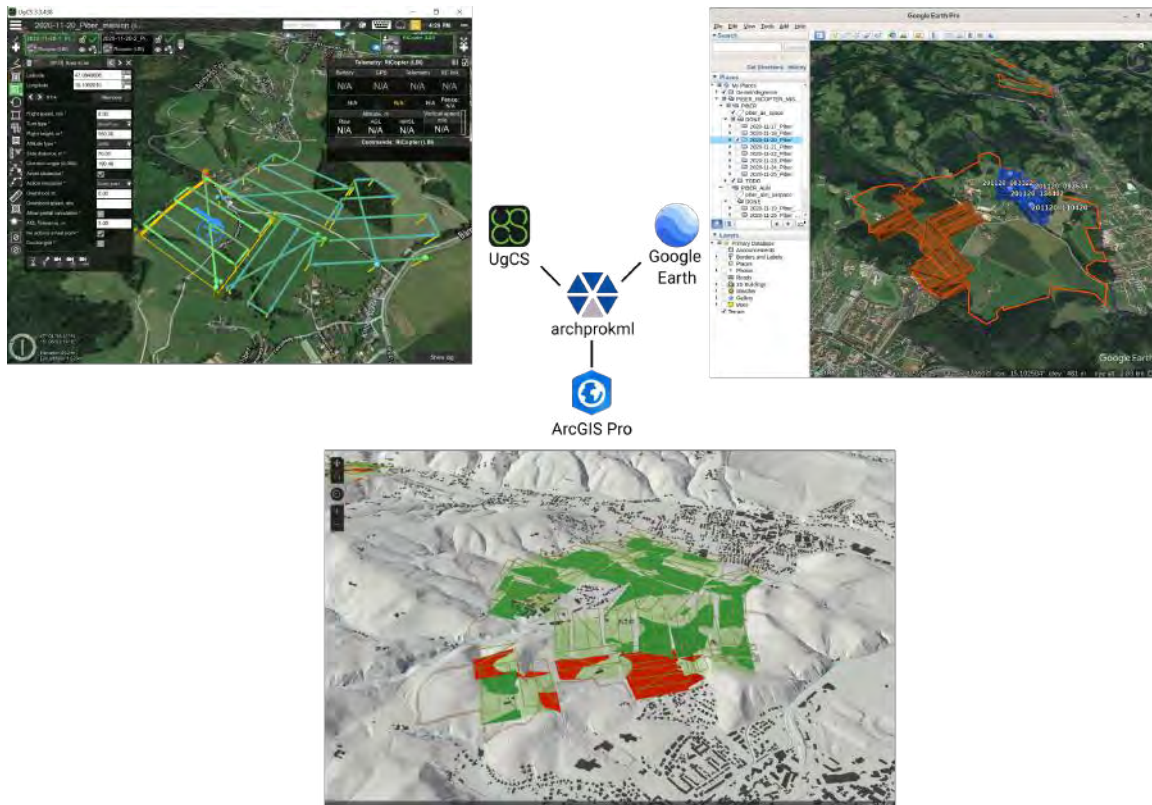
Fig. 26. The archprokml tool allows to convert KML files from one tool into another.
