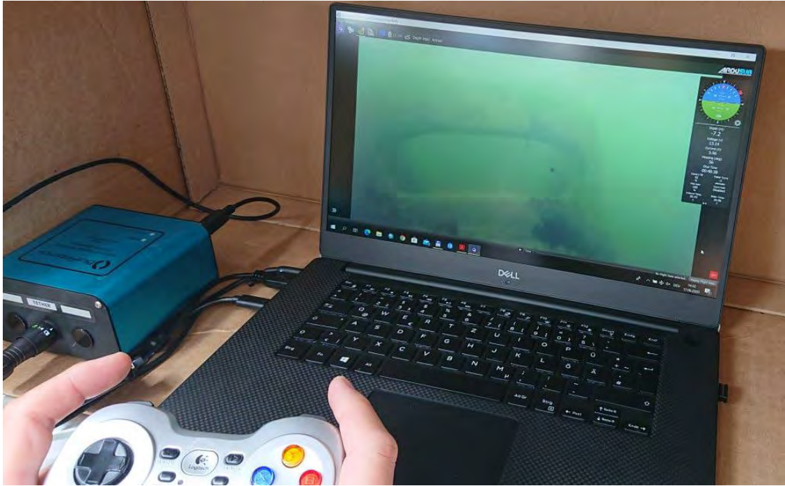
Fig. 37. The rear of the car wreck filmed at a depth of 7.5 m by the BlueROV2 that is steered with an X-Box controller.
