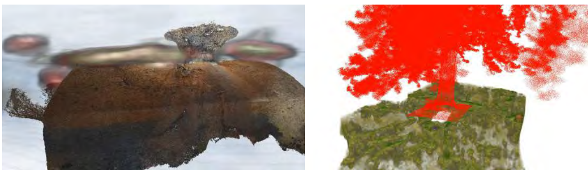
Fig. 32. Integrated point cloud rendering. Conjoint visualisation of a GPR datasets of an Etruscan grave in Cerveteri (Italy) together with the inner surface of recorded data using a laser scanner (left). This outside view shows how well the point cloud surface matches the ceiling of the grave made of large stone blocks – red and green regions in the GPR visualisation. The image on the right shows an application combined GPR/point clouds visualisation beyond archaeology. An uncoloured laser scan of a tree complements its roots that are visualized based on GPR data.
