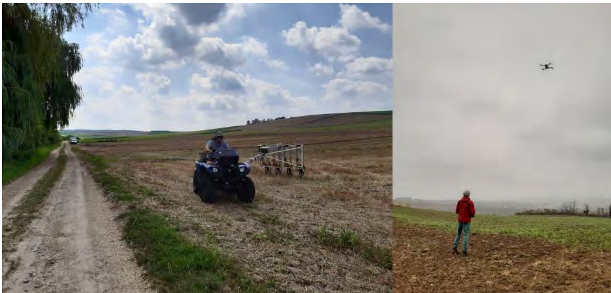
Fig. 7. Surveys at the Dernberg with magnetometry (left) as well as a the RiCOPTER UAV (right).
