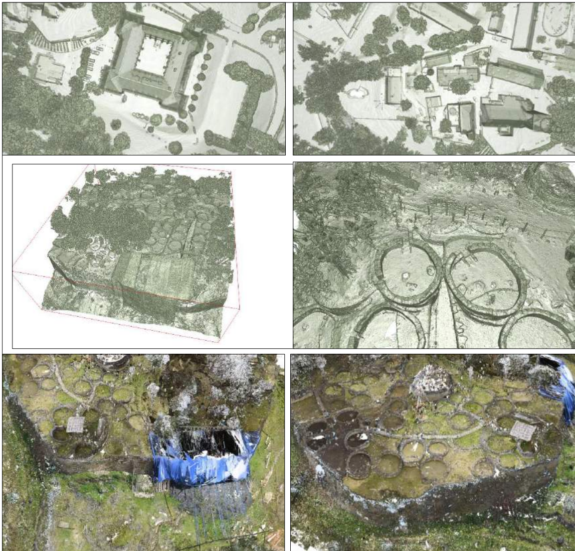
Fig. 12. Big data visualizations: High-resolution 3D point cloud from the Lipizzaner stud Piber, Styria recorded using a 3D laser scanner mounted on a drone. For semi-transparent visualization the point cloud was converted into a 3D density volume representation (top). High resolution point cloud visualizations from ALS dataset from Kuelap, Peru including colour information (center and bottom).
