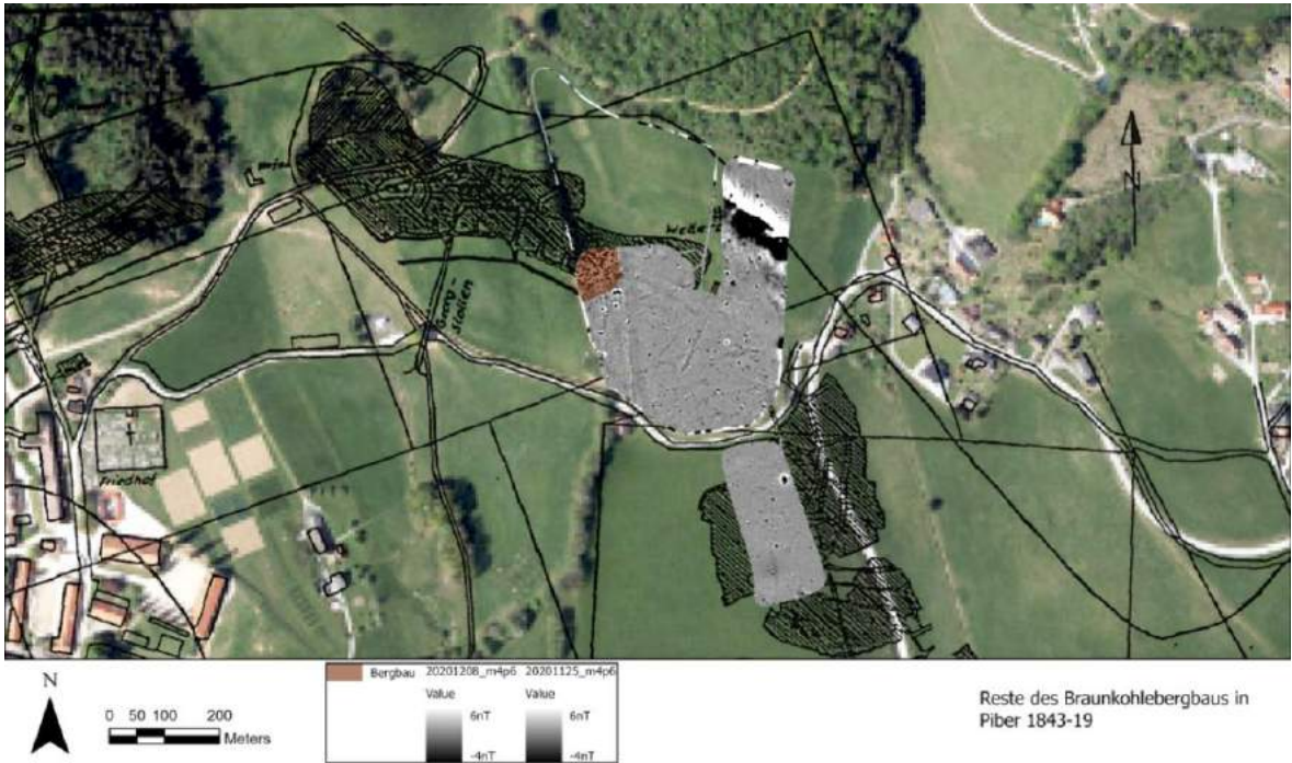
Fig. 18. Overlay of the geomagnetic data with the historic mining map of Piber.
