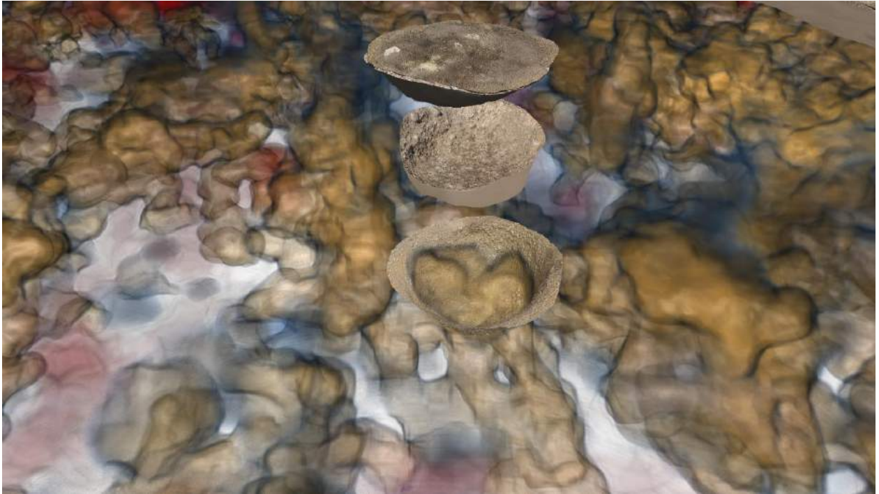
Fig. 10b. Detail view of the same scenario showing good correspondence between a GPR feature of high reflectivity in the center of the arena and a pit filled with stones in the excavation.
