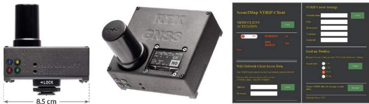
Fig. 64. The new RTK-enabled GNSS-IMU logging device (left and middle) with the interface controlling its settings (right).
