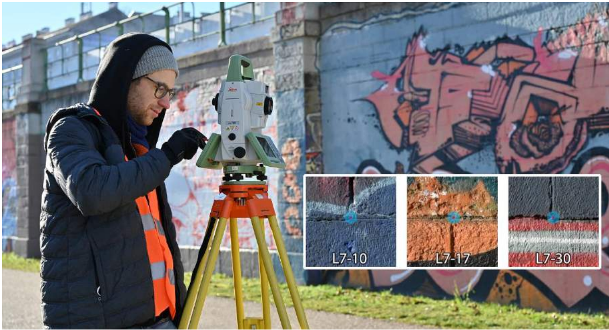
Fig. 66. Benjamin Wild operating the Leica Viva TS16 total station. The inset on the lower right displays three typical GPs.
