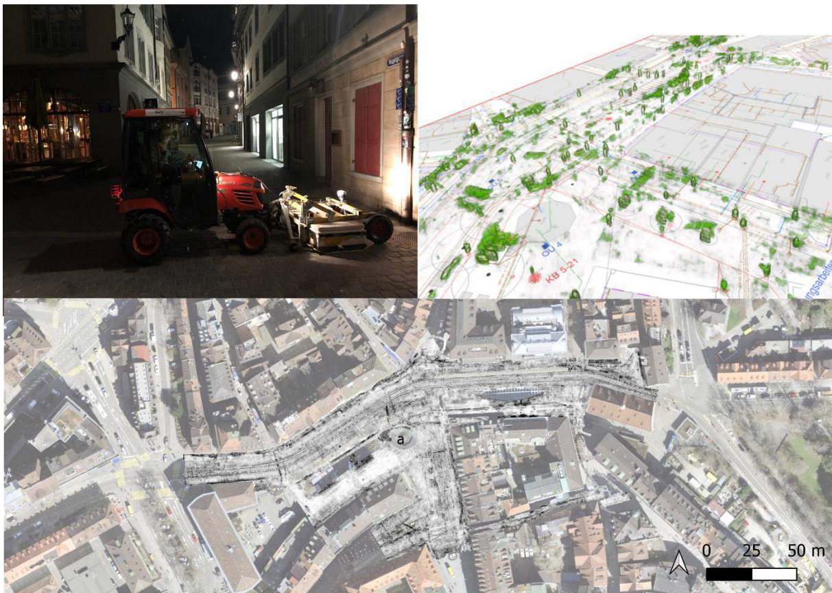
Fig. 6. From left to right: 16 channel MÅLA Mira antenna array in operation in the historic city centre of St. Gallen. Analysis of sewer shafts and installations with ArchProspector 3D, view from south-west. Greyscale-image of GPR data, depth slice 40 - 80 cm (the letter “a” marks a round pavilion).
